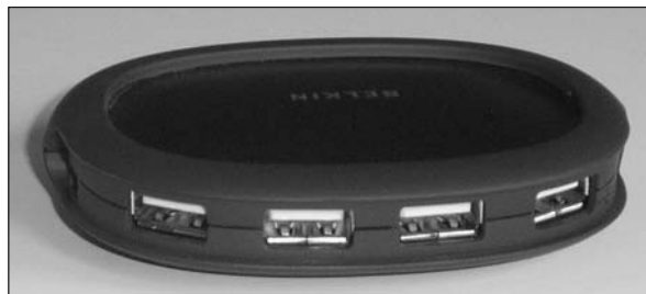
Figure 1-19: A USB hub with four ports.
