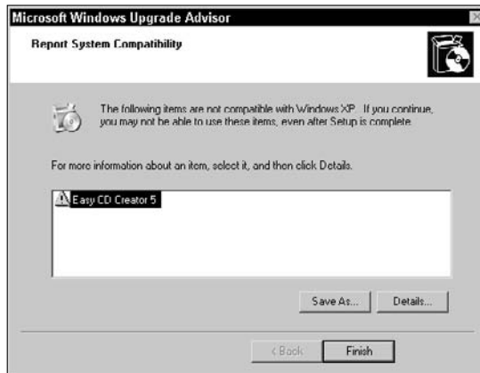
Figure 3-33: The Upgrade Advisor identifies known hardware and software issues when upgrading to Windows XP.
