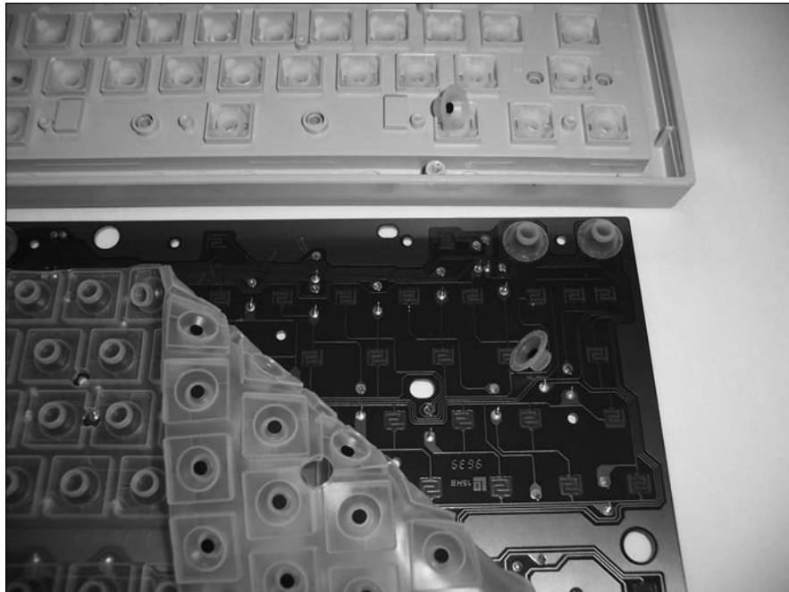
Figure 2-6: Keyboards can be taken apart and cleaned, but they do contain a lot of little components.
