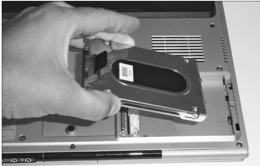
Figure 7-9: Replace the hard drive on a laptop for more storage.
