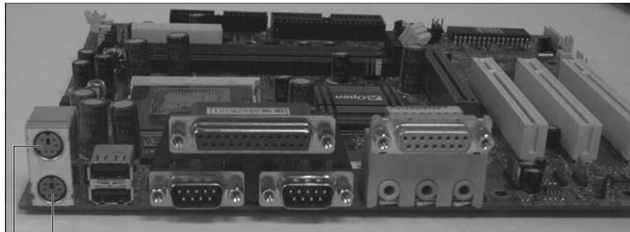
Figure 1-15: PS/2 connections for a keyboard and a mouse.
