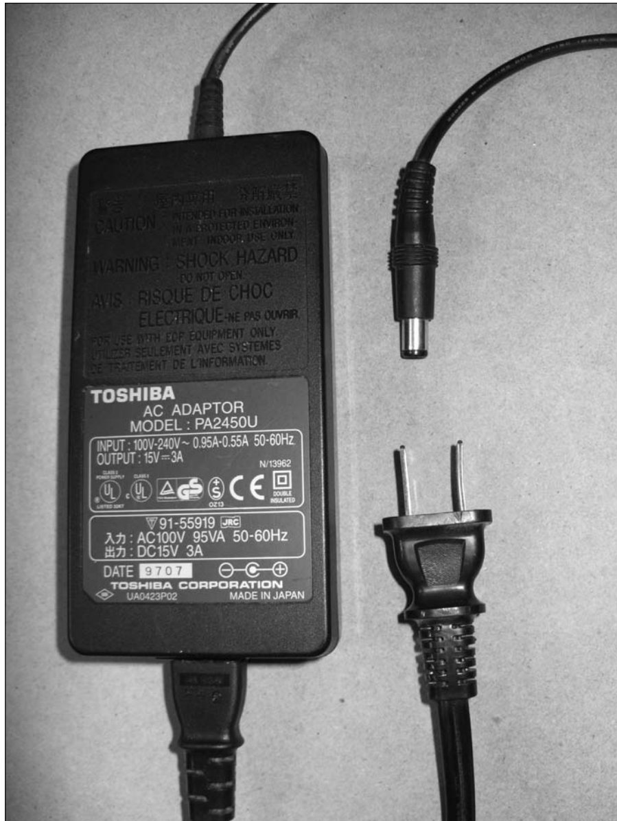
Figure 6-3: An AC power adapter for a Toshiba laptop.
