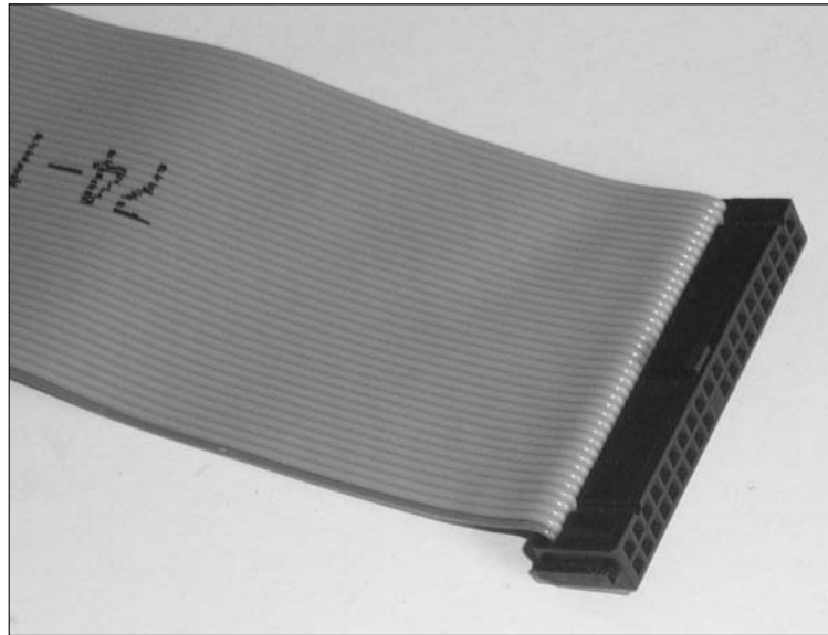
Figure 1-25: A 40-wire IDE ribbon cable.
