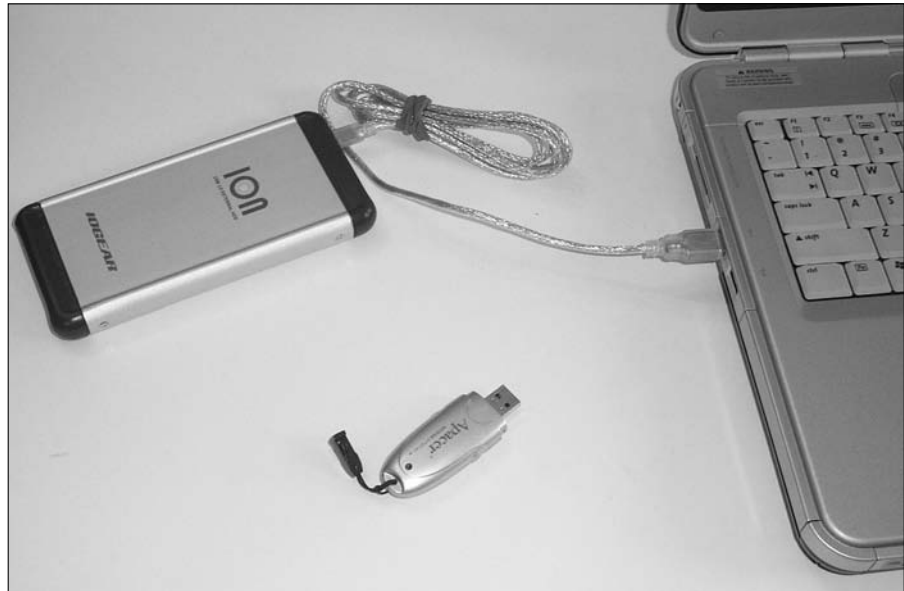
Figure 7-10: Add storage space by using a USB external hard disk (top) or a USB flash drive (bottom).
