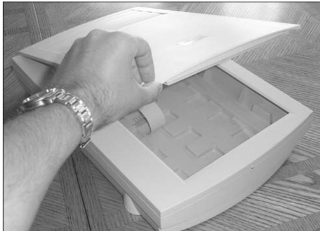
Figure 6-1: A flatbed scanner uses a scan head that moves under the object being scanned.
