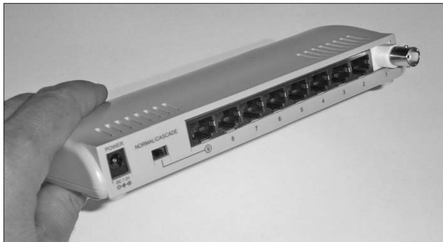
Figure 1-25: A network hub with eight RJ-45 ports and one BNC port.
