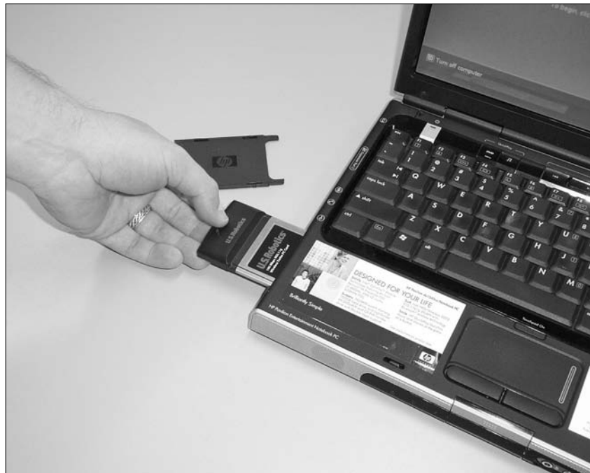
Figure 7-7: Inserting a PCMCIA card into the PCMCIA slot.
