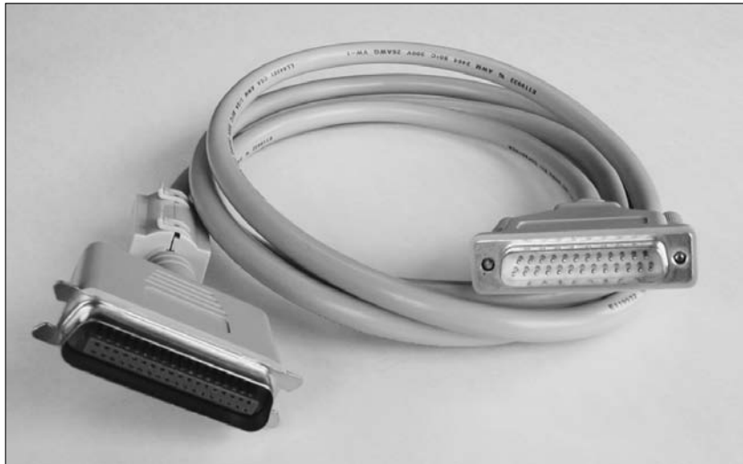
Figure 5-6: A parallel cable uses a 25-pin/36-pin connector on either end of the cable.
