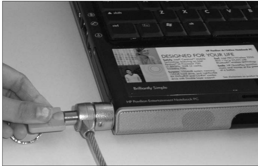
Figure 1-5: A lockdown cable is used to secure computer equipment to a desk.
