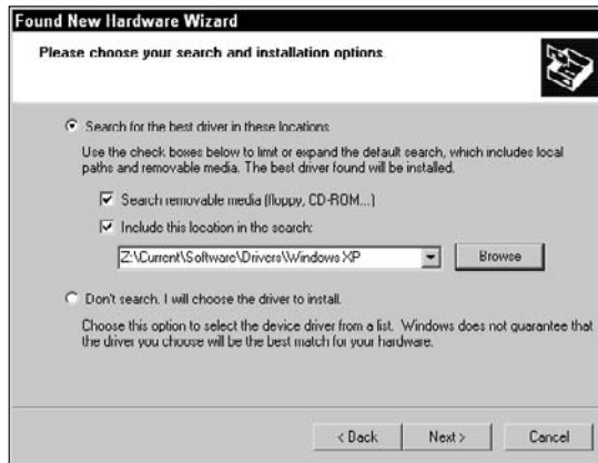
Figure 1-2: Plug and Play detection is used to initially locate all devices on your computer.
