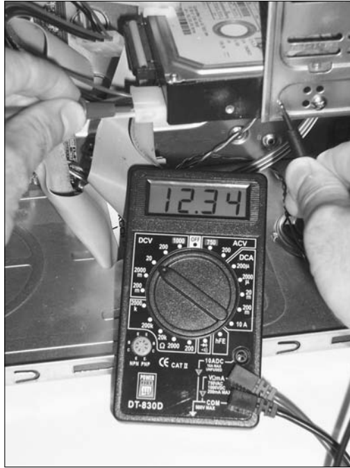
Figure 2-9: Back-probing power connectors is a standard method for testing power in systems.
