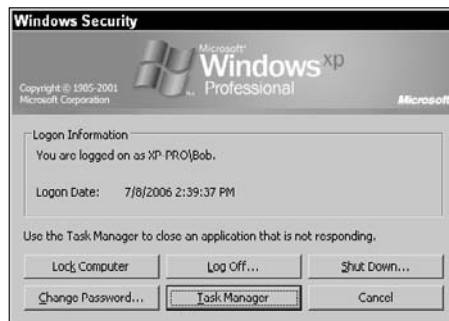
Figure 2-4: Use the Security dialog box in Windows XP to launch Task Manager.
