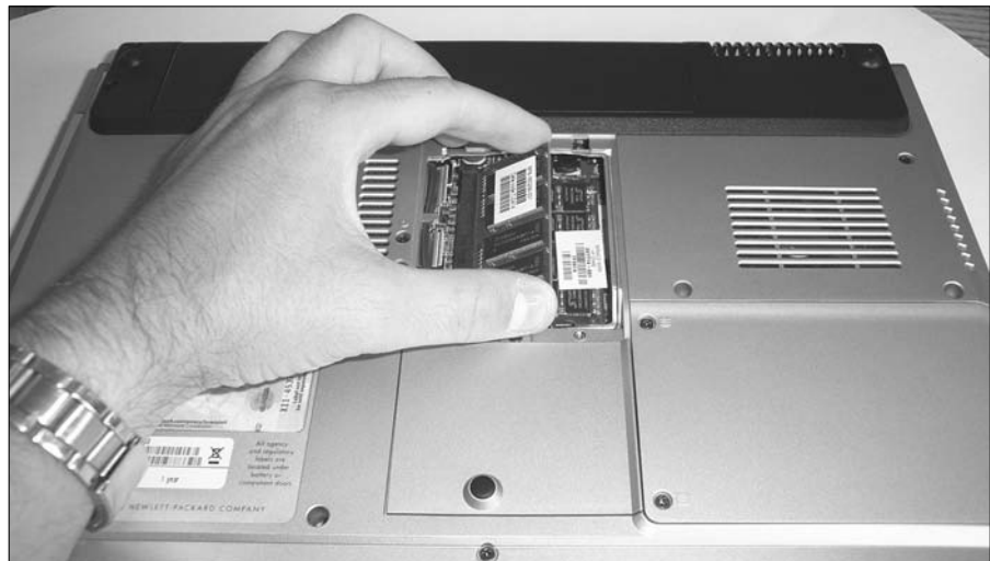
Figure 7-8: Install a SODIMM into the laptop to add more memory to the laptop.
