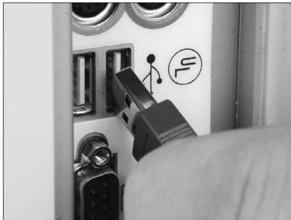
Figure 5-7: A USB connector is a popular method today to connect printers to computers.
