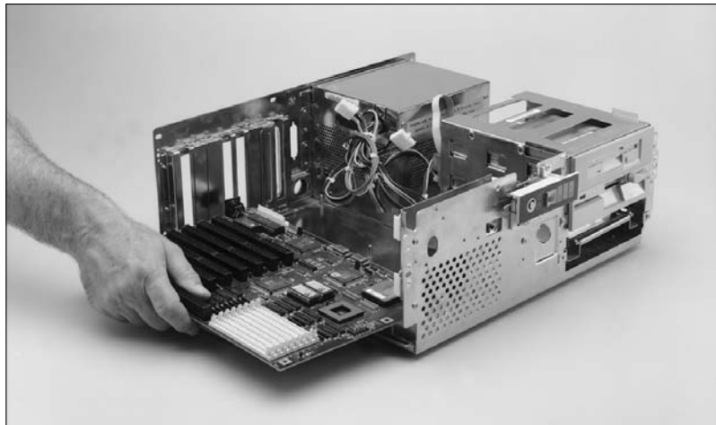
Figure 1-30: A full AT mother- board in a full AT case.
