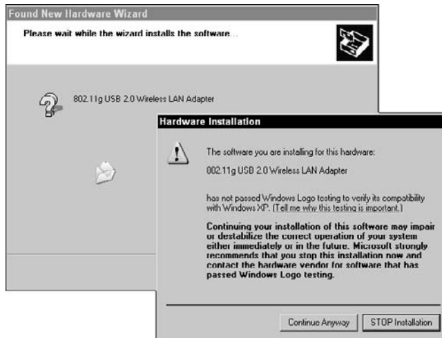
Figure 1-7: Driver signing prevents installation of unwanted drivers.
