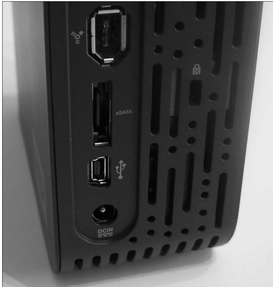
Figure 5-20: An eSATA connector on an external hard drive.
