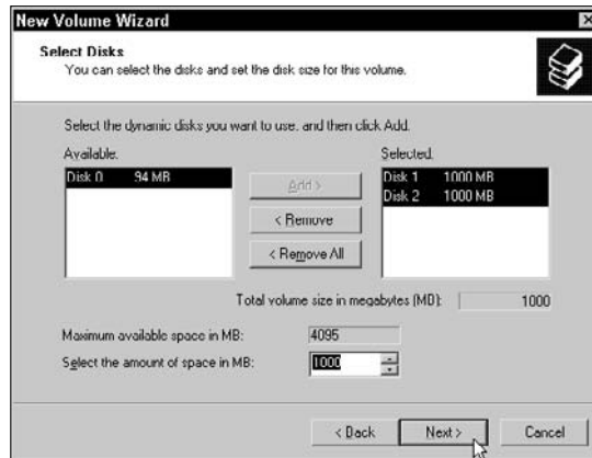
Figure 5-39: Selecting the disks for the mirrored volume and setting the volume size.
