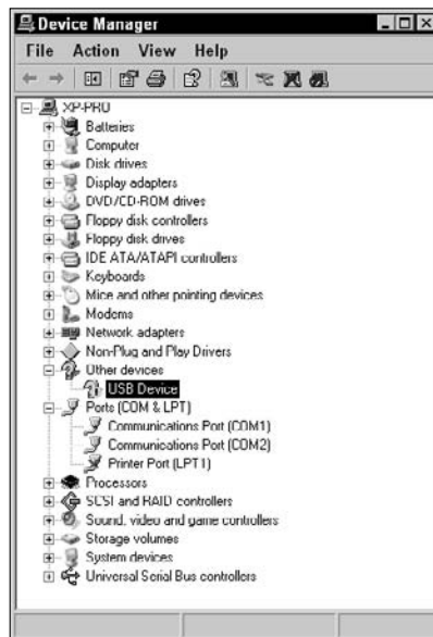
Figure 4-12: When looking for malfunctioning devices, look for the warning symbols like the one next to USB Device.
