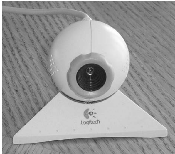
Figure 6-5: A webcam captures live video and sends it to anyone you are conferencing with.
