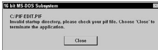
Figure 2-6: Notification for working directory that does not exist.
