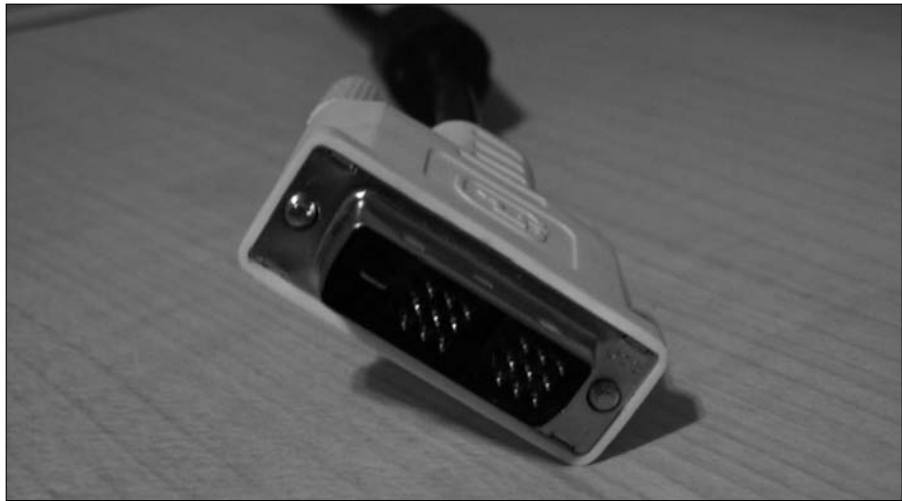
Figure 3-2: Looking at a DVI-D connector on a DVI cable.
