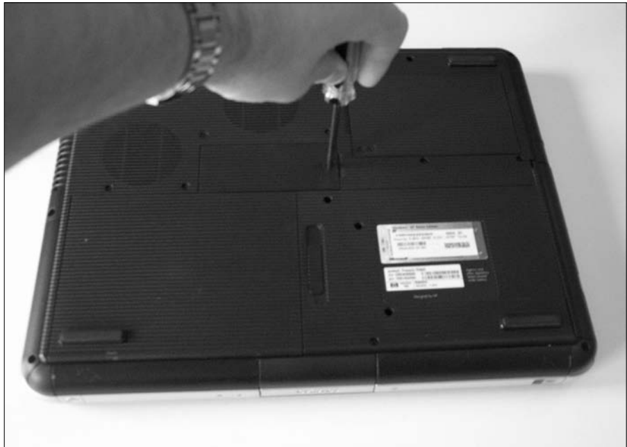
Figure 3-8: Remove the cover to add memory to a laptop.
