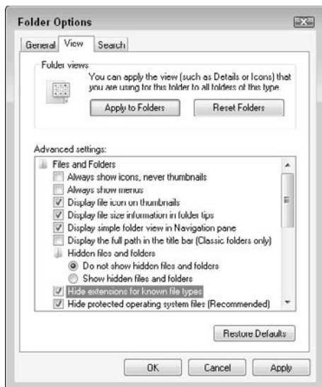
Figure 4-8: You can tweak your Folder Options to display file extensions on your files.
