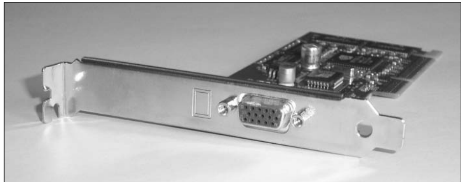
Figure 3-1: Looking at the back of a video card and the port style.
