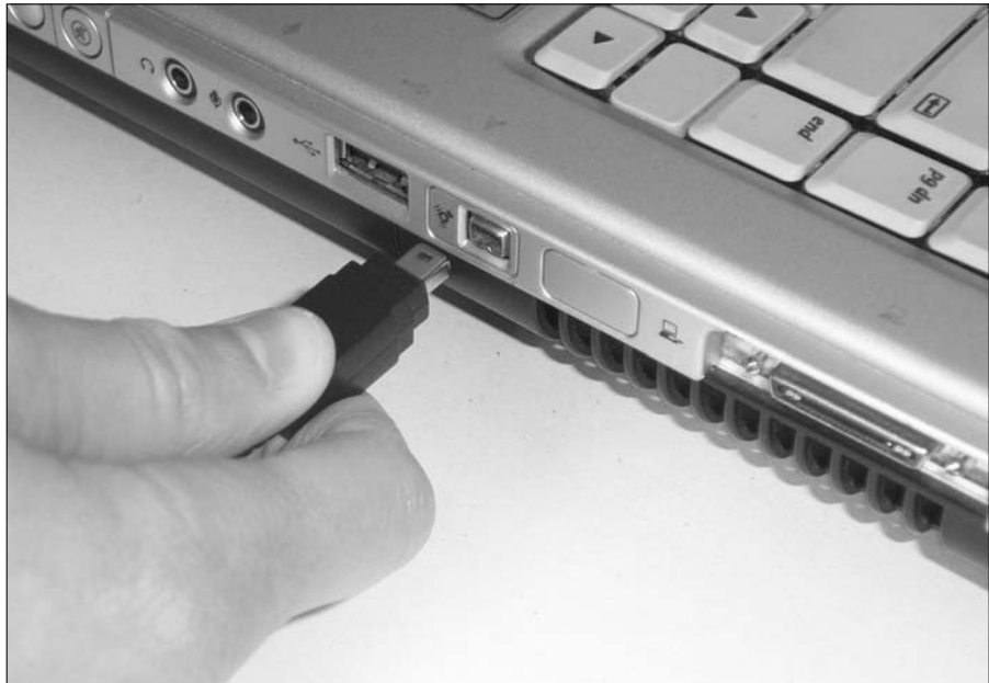
Figure 1-20: A digital video camera being connected to a system by the FireWire port.
