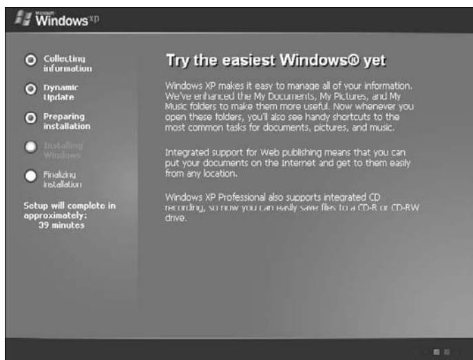
Figure 3-19: The GUI-mode setup phase of the Windows XP installation.
