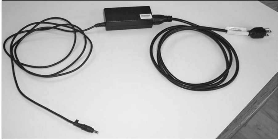
Figure 7-5: An AC adapter supplies power to the laptop and charges the battery.
