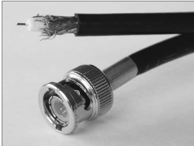
Figure 1-11: Looking at coaxial cable and a coax cable with the BNC style connector.
