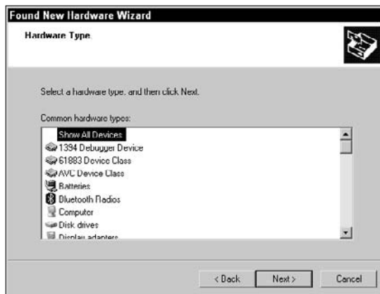
Figure 1-3: Choose the type of device you are installing so that you can look at a filtered list.
