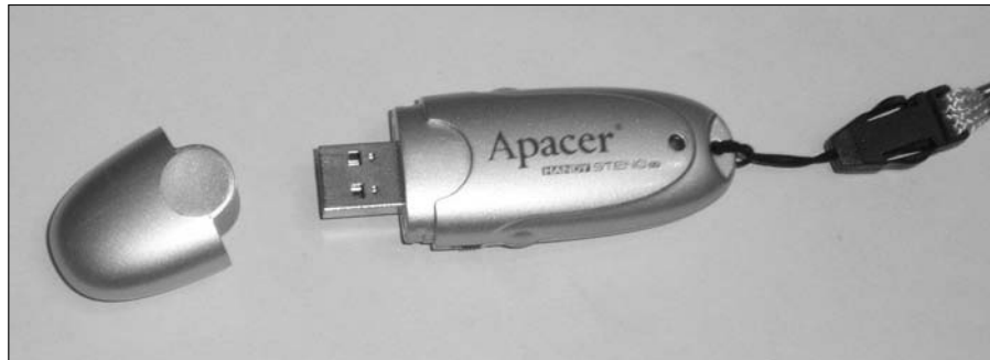
Figure 5-21: A flash drive uses a USB connection to interface with the computer.
