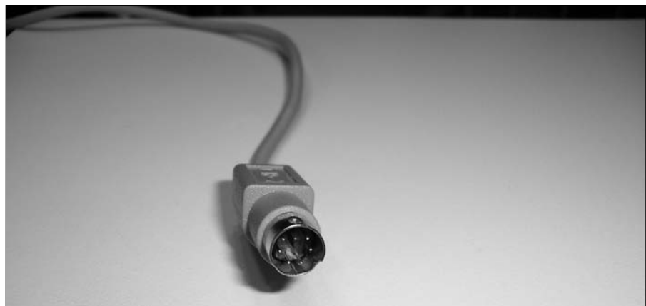
Figure 1-11: PS/2 (mini- DIN 6) connectors are used for keyboards and mice.
