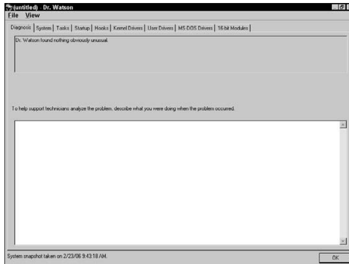
Figure 1-1: Dr. Watson provides the Diagnosis tab for you to describe what you were doing when the error occurred.
