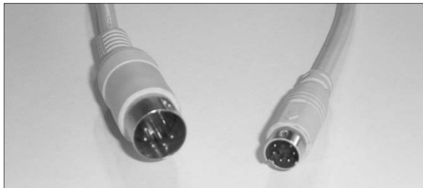
Figure 2-3: A DIN-5 connector (left) beside a PS/2 keyboard connector (right).
