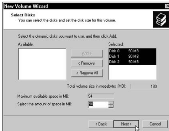
Figure 5-43: Select the disks to be members of the RAID 5 volume and specify the size of the volume.
