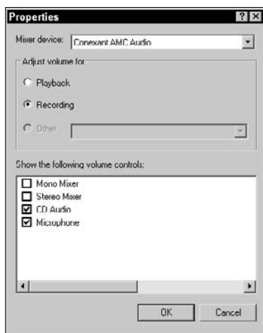
Figure 6-6: Ensure that the microphone is set as a recordable device.
