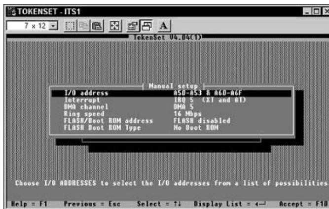
Figure 4-15: Changing resources on a non-Plug and Play device using the setup disc.
