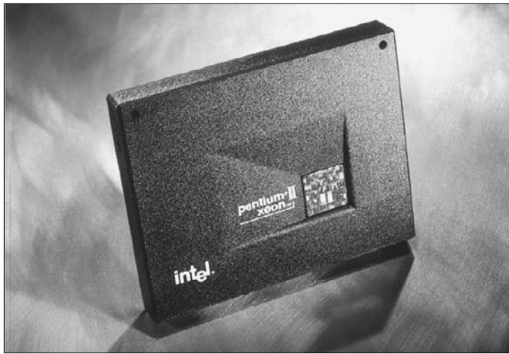
Figure 2-13: The Pentium II Xeon processor was originally delivered in the SEC package.
