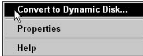
Figure 5-28: Converting a basic disk to a dynamic disk.
