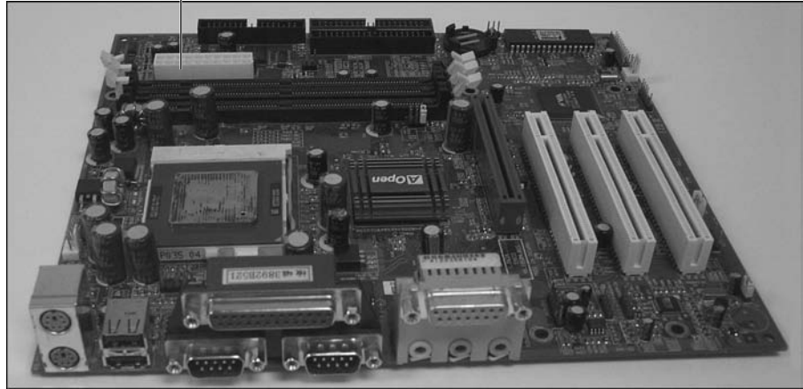
Figure 1-22: The ATX power connector on an ATX motherboard.
