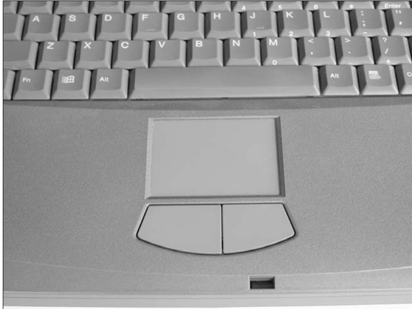
Figure 2-11: A touch pad is a popular input device to control the mouse pointer on a laptop computer.
