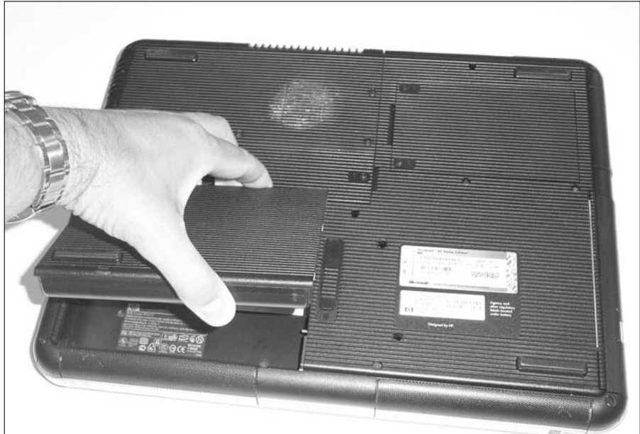
Figure 7-2: Replacing a battery on a laptop system.
